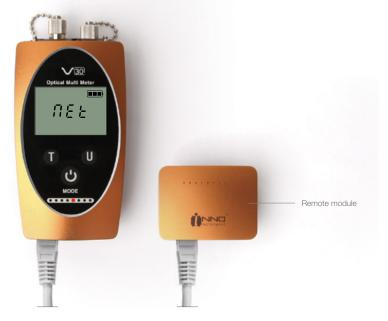
The "Network cable/ phone line test" (NET) function is used in network generic wiring and for verifying the link on-off condition of network including the sequence of testing cable connection systems. Test will begin when this NET function is enabled; the 8 indicators are used for indicating the sequence of testing cable connection systems. When the network cable or phone line is connected to this instrument and remote model. 8 indicators will blink in turn.
