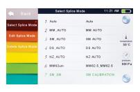
Selected splice mode appears on the screen. Press [RESET] button to return to initial interface page.
