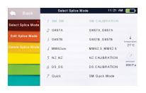
Selected splice mode appears on the screen. Press [RESET] button to return to initial interface page.
