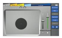
Fiber end tester (peripheral required) is mainly used to test the cleanliness and flatness of the fiber end face.
